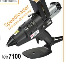
Very high output pneumatically assisted extrusion glue gun for industrial use. Air assisted output reduces operator fatigue. Power on indicator and speed load design helps save time reloading. Requires air and electric supply. Maximum 7 bar (100psi), for best results set to 4-6 bar (60-90psi) dependent on output requirements.
