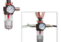
Pressure regulator, filter and water separator enables you to control the output of the glue gun and extends tool life.
